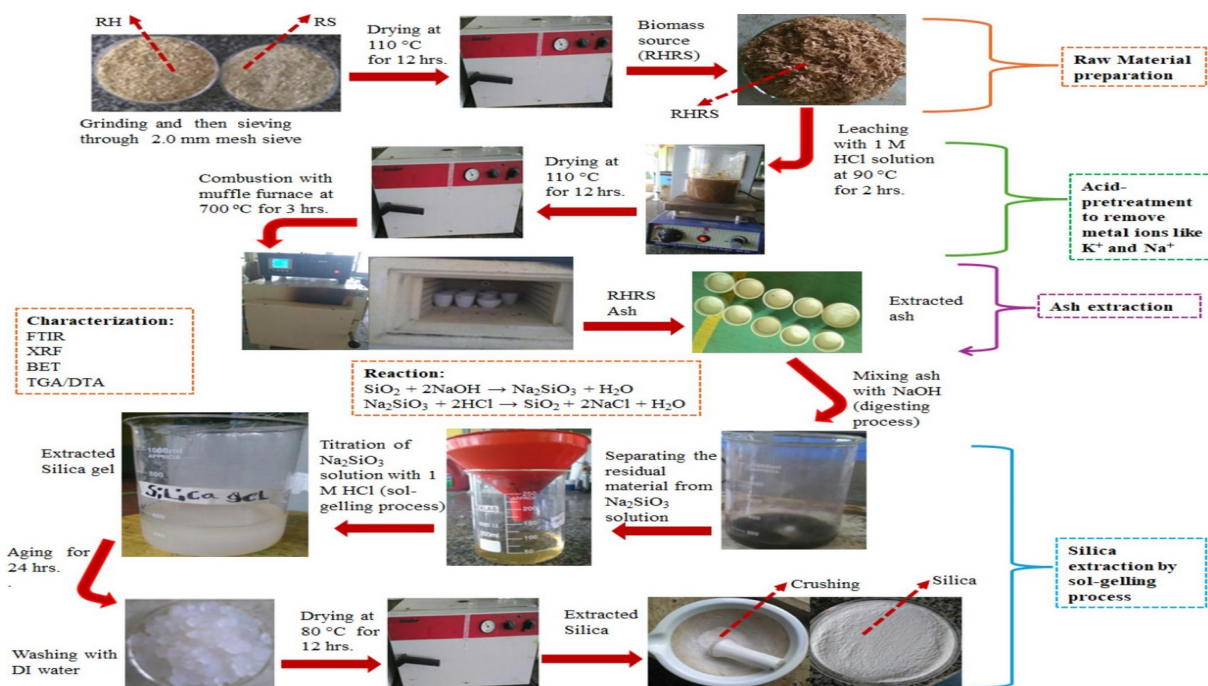
1-rasm. Guruch qobig'idan SiO 2 olishning prinsipial texnologik sxemasi
